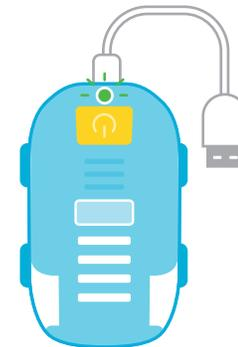
The LED will turn green when the battery is fully charged.
